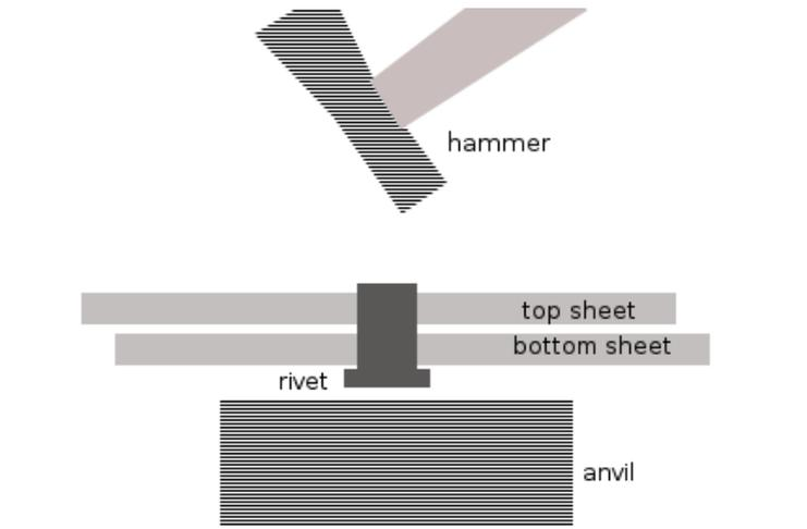
Riveting works well for metals and materials such as vintage pieces which can't be soldered. It also can allow for joints to be flexible or articulated. To have solid joint use two or more rivets, for a moving part use one rivet to allow the components to swivel.
